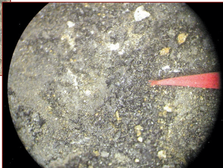
Figure 6. Localized crushing of the asphalt flood coating at the point of impact is shown in this 10-power photograph.
