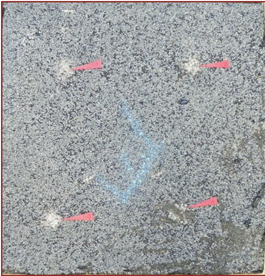
Figure 25. Aged modified bitumen roof on the noninsulated substrate after the sample was impacted by the four missile drops.
