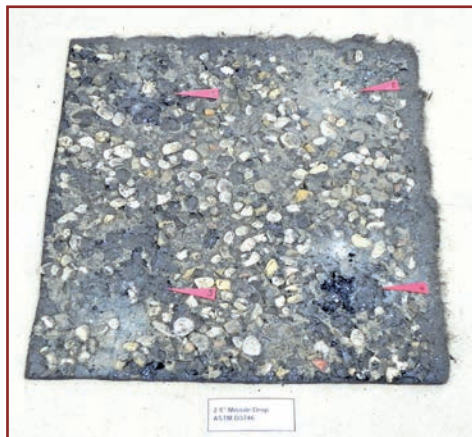
Figure 4. The test sample after the missile drop and after the loose gravel was removed.
