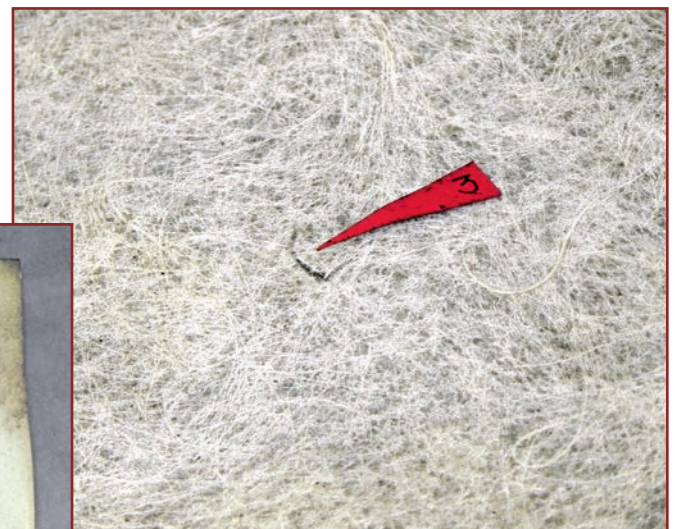
Figure 24. Fracture in the bottom ply (fiberglass felt) on the noninsulated sample.
