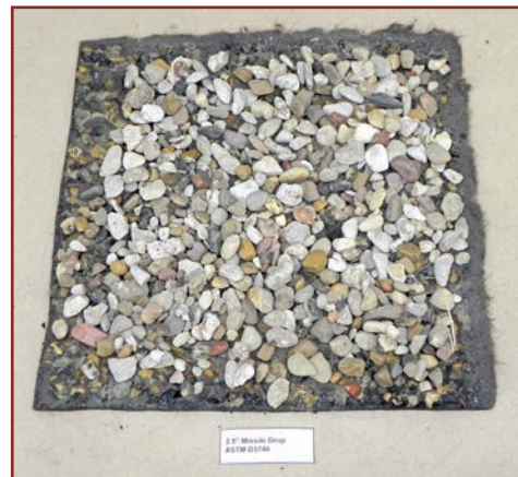
Figure 3. The test sample before the missile drop.
