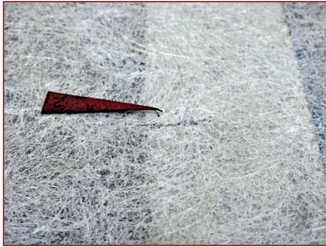
Figure 41. Fractured bottom ply of the membrane.
