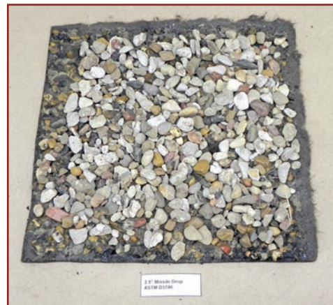
Figure 3. The test sample before the missile drop.
