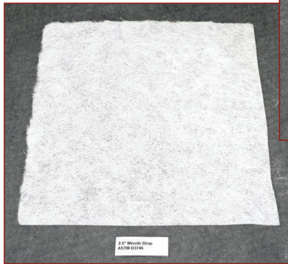
Figure 14. Desaturated bottom ply of felt in the noninsulated (firm substrate) sample.
