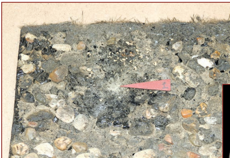
Figure 5. The test sample after the missile drop showing crushed gravel at point of impact.
