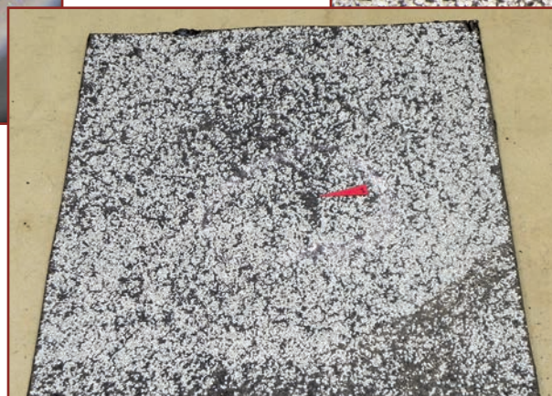
Figure 33. Test sample from a modified bitumen roof with an area of localized granule loss at the point of interest noted.
